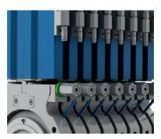
Slitting widths from 19 mm with the nested model
