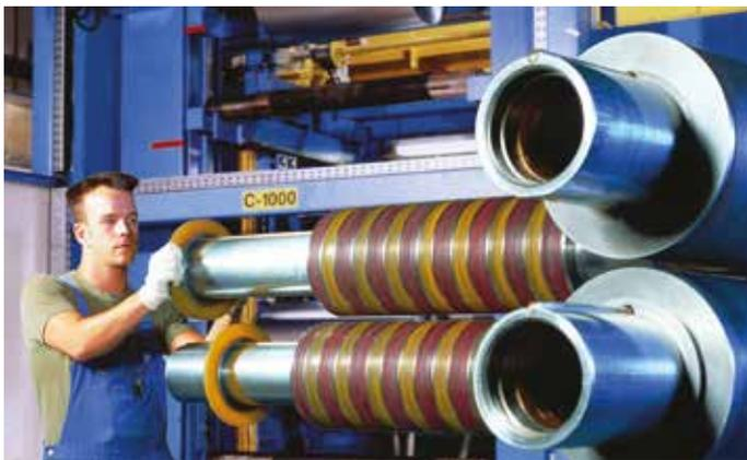
To optimise cutting production and minimise set-up time of knife shaft systems, a new computer program is available to DIENES customers. After setting a pre-determined cutting plan, the program accurately defines the proper sequence for mounting cutting tools. The results are cost savings when minimum time is required to assemble tooling and test cuts during set-up are not required.
